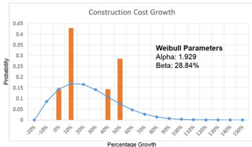
Figure 16 – Construction Cost Growth Actuals and Fitted Weibull
