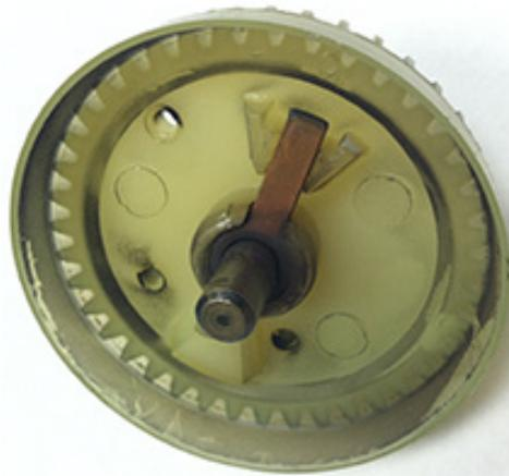
**Figure 3. Affected K3008 Distributor Gear With Copper Electrode**
