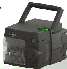
The shoebox-sized Axcend Focus LC is a lightweight HPLC designed for both field and laboratory use.
